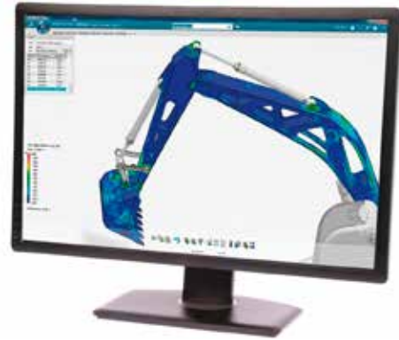
Backhoe arm mechanism arm actuation model analyzed with Structural Performance Engineer to optimize product design
