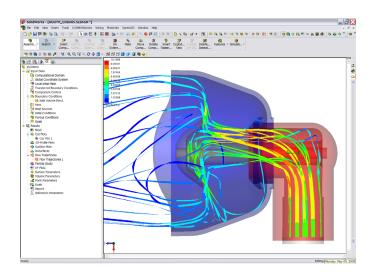
SOLIDWORKS Flow Simulation enabled engineers to determine the optimal design for a new oxygen delivery device.
