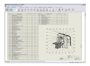
With SOLIDWORKS software, you can automatically generate a bill of materials, which you can export as an Excel spreadsheet or in other formats for import into MRP systems.
