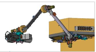
Using SOLIDWORKS software, ASI engineers developed the robotic arms for NASA's Mars Exploration Rover (MER) mission, which provided the first opportunity for detailed scientific studies on the Martian surface.
