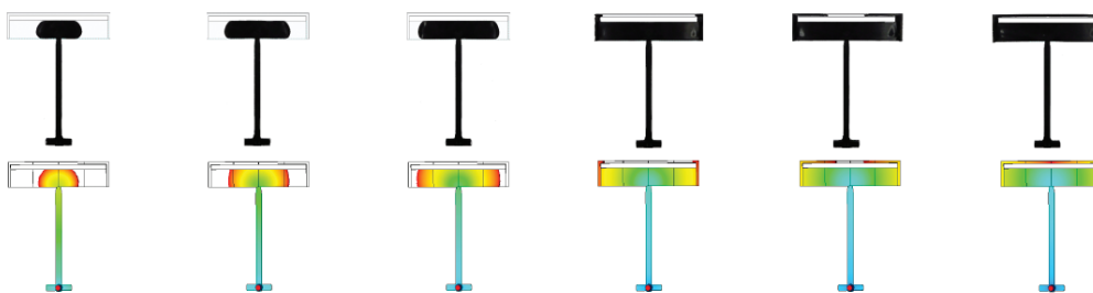
Bow Model - Short Shot Series Fill Pattern Comparison
