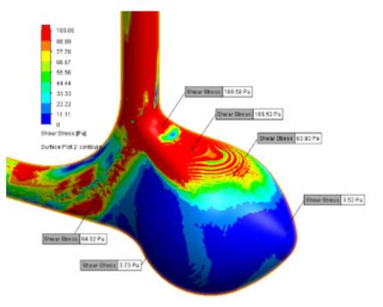
Tiniko was able to connect their data from SOLIDWORKS to perform multi-step analysis using **3D**EXPERIENCE Works Simulation.
