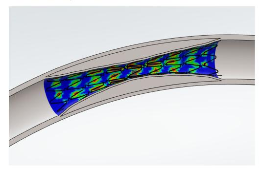
Special surface capabilities within **3D**EXPERIENCE Simulation tools help to represent stent contact with catheters, balloons and arteries in both straight and curved conditions.
