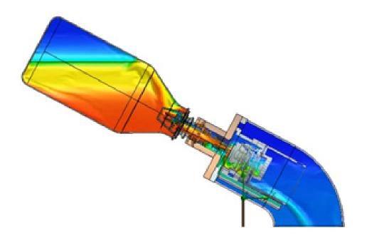
GE Healthcare optimized the liquid and gas exchange paths when transferring an anesthesia agent from a sealed bottle to its vaporizer using the free surface capabilities in SOLIDWORKS Flow Simulation
