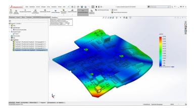
Thermal analysis calculates the temperature and heat transfer within and between components in medical design and its environment.
